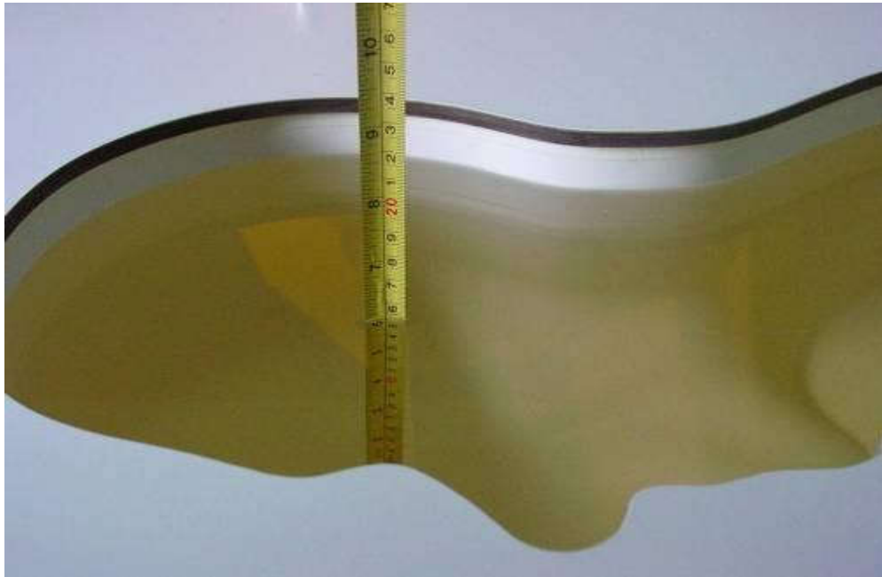
Picture 7-1: Liquid depth in the Head Phantom (750MHz)
