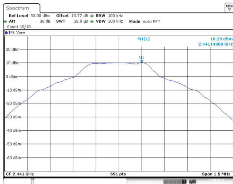
Fig. 16 Conducted Spurious Emission (GFSK, CH39, 2.441GHz)
