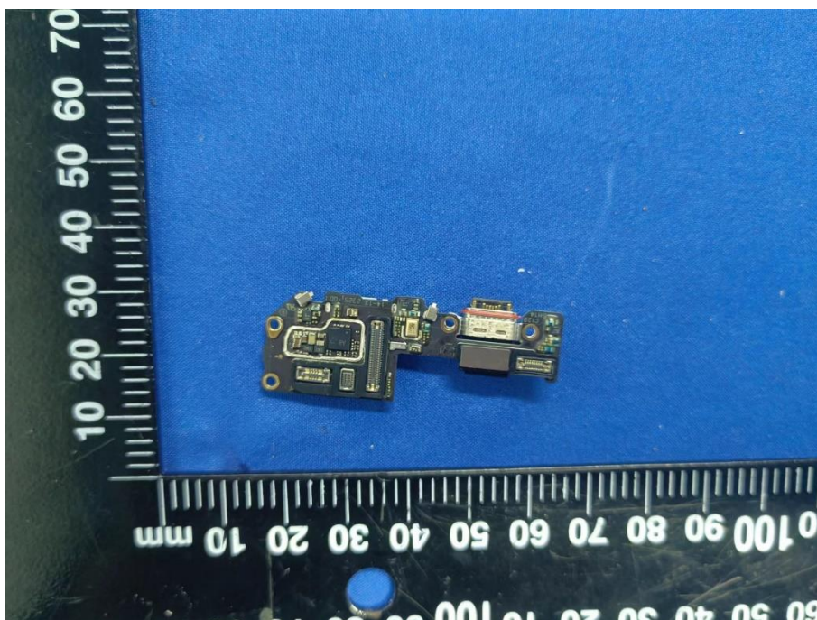
SECONDARY BOARD REAR VIEW (WITHOUT SHIELDING)
