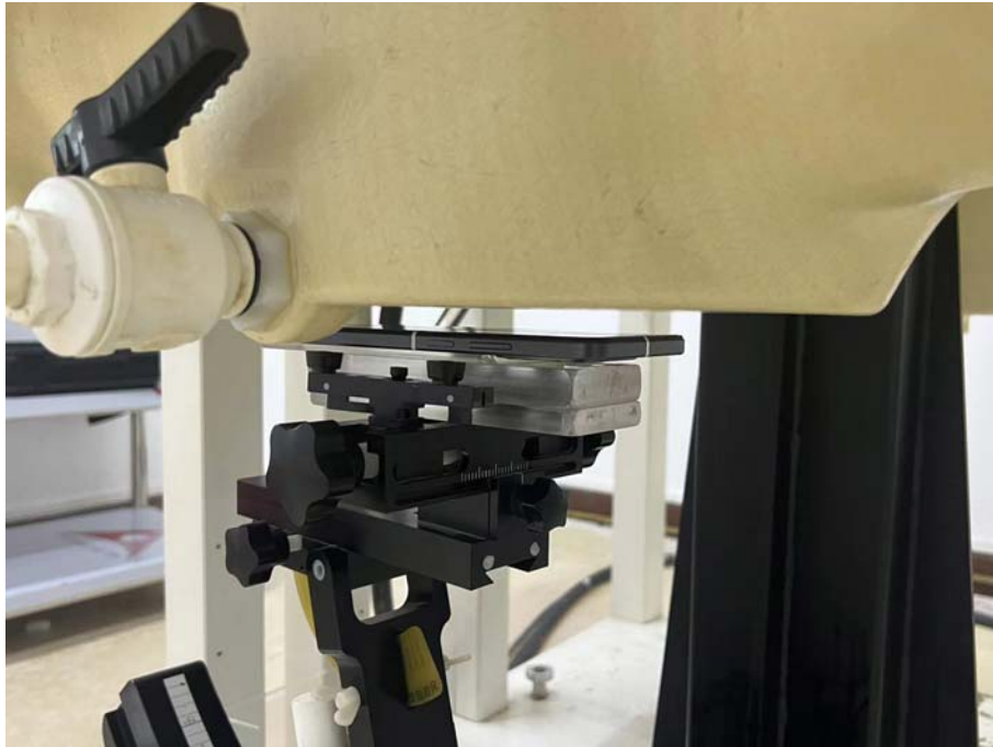
Front Side (Test distance: 10mm)
