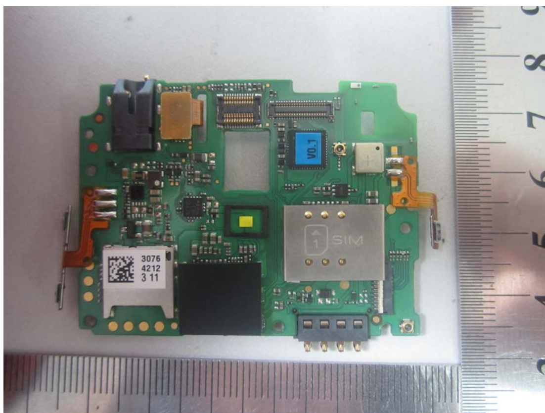
2. Mainboard front view with shielding
