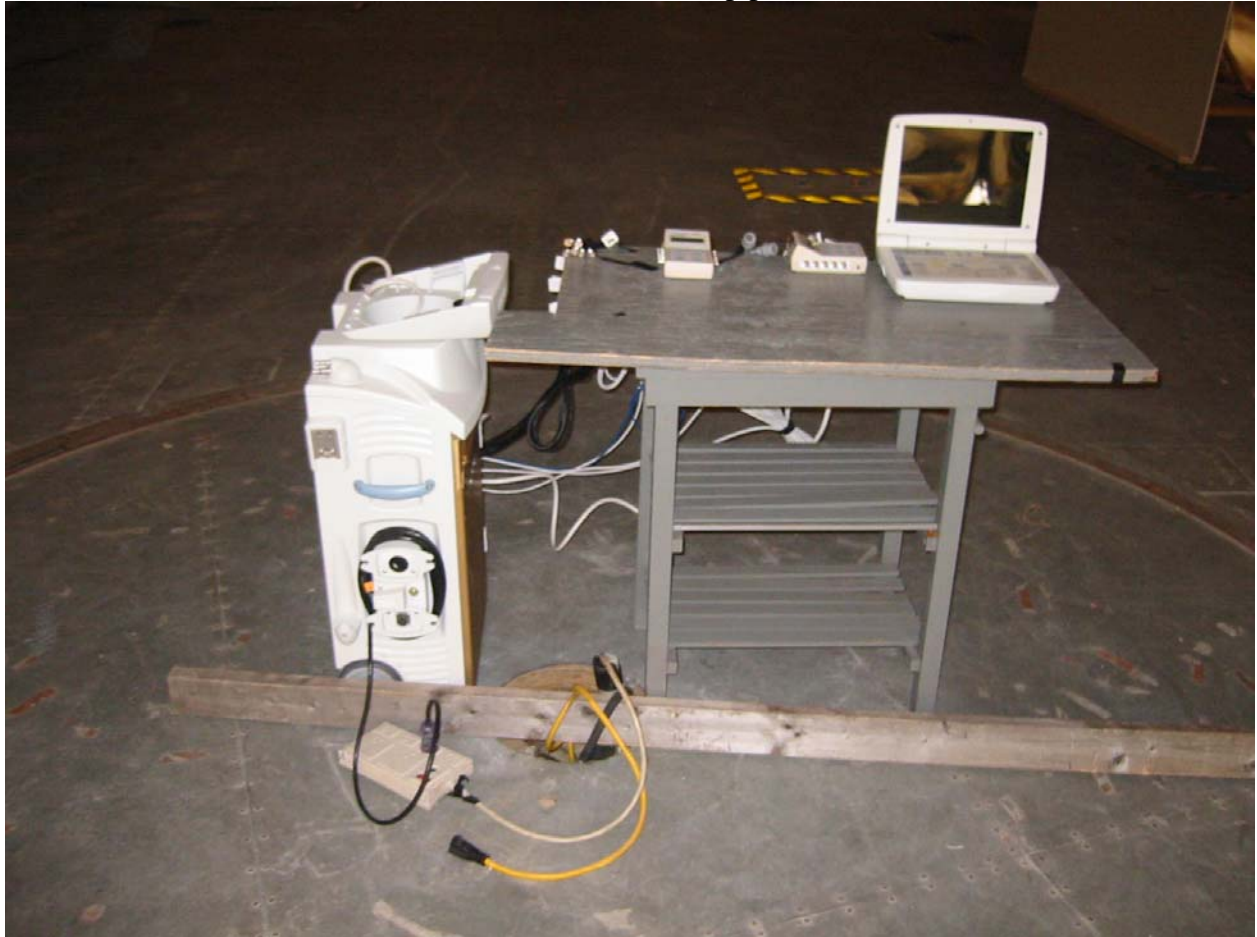
Radiated emissions setup photos
