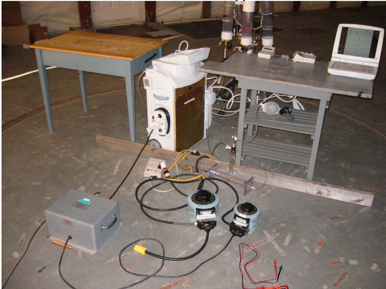
Line-Conducted Emissions, Front View, Ventricular Assist Mode
