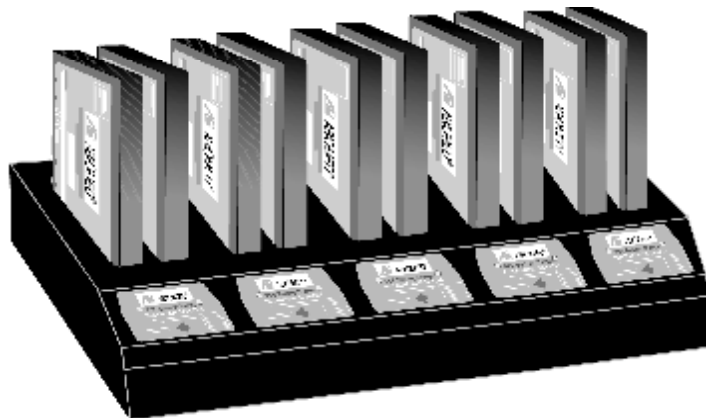
Figure 4.29 Charging the Used Batteries
