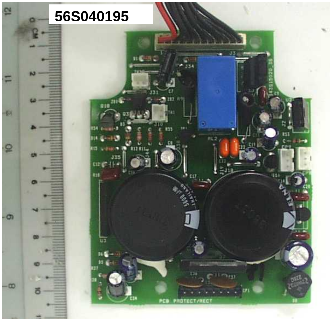
Rear Left/Right Speaker – Rectifier Board Component Side
