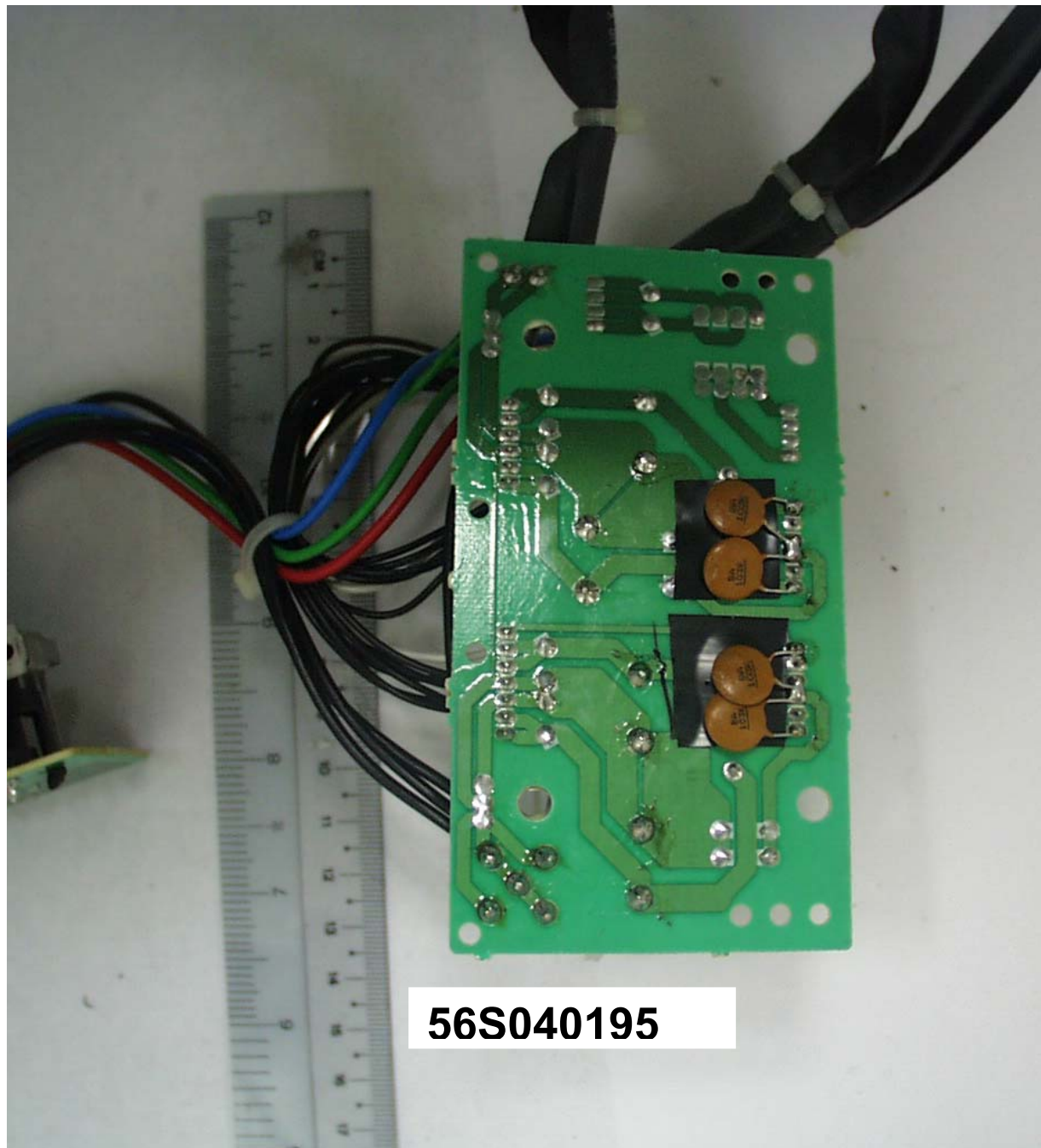
Subwoofer – Power Supply Trace Side
