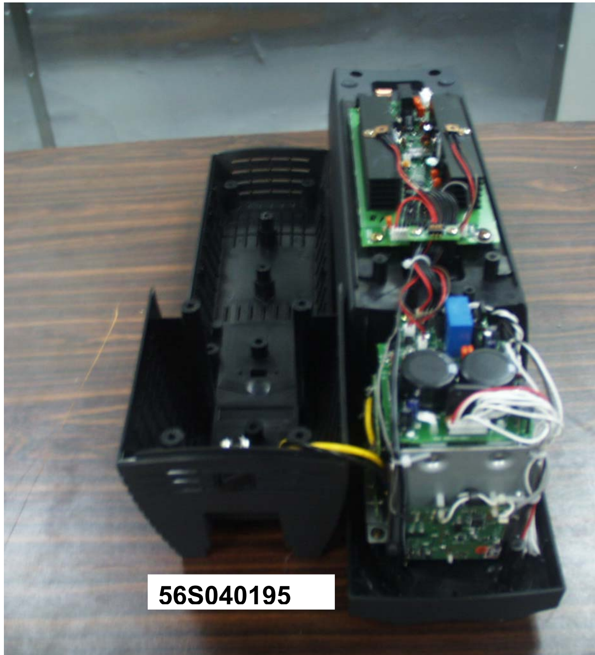
Rear Left/Right Speaker – Internal Layout
