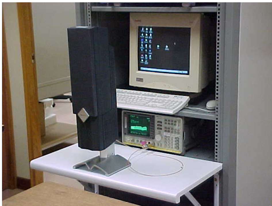
Number of Hopping Frequencies Measurement Test Setup – Wireless Speaker
