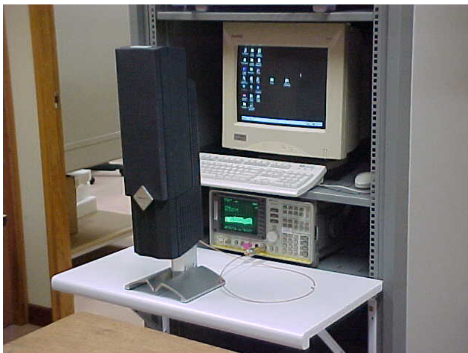
Peak Power Spectral Density Measurement Test Setup – Wireless Speaker
