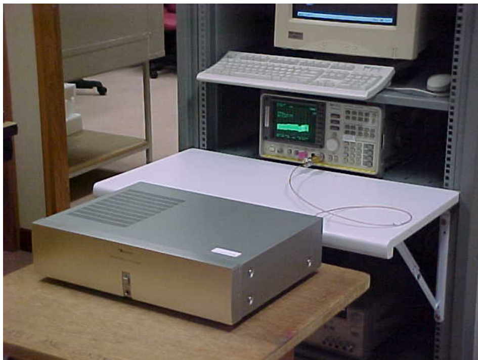
Peak Power Spectral Density Measurement Test Setup – AV Unit
