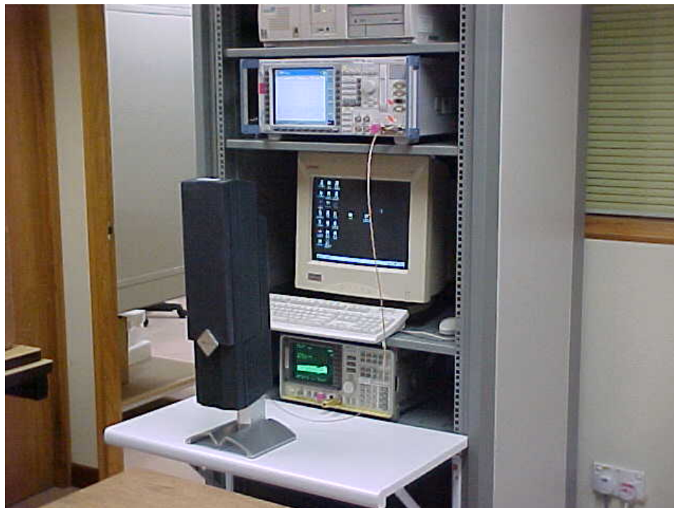
Maximum Peak Power Measurement Test Setup – Wireless Speaker
