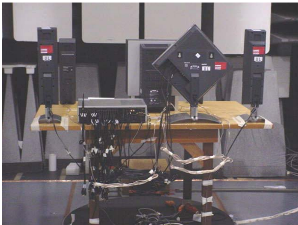
Radiated Emissions Setup (Rear View)
