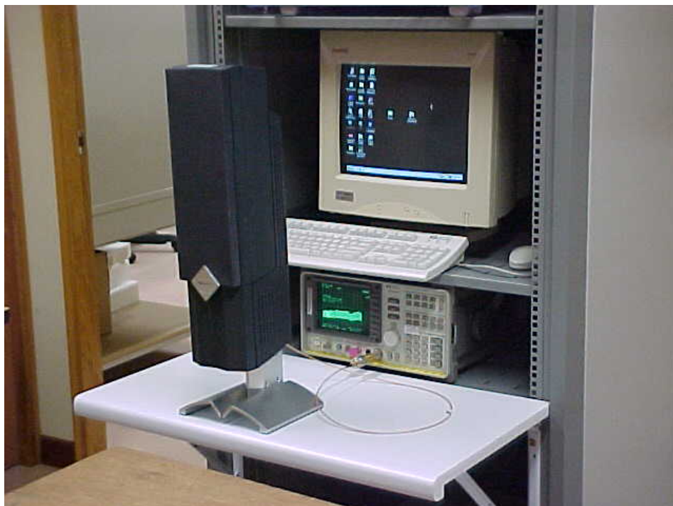
Carrier Frequency Separation Measurement Test Setup – Wireless Speaker
