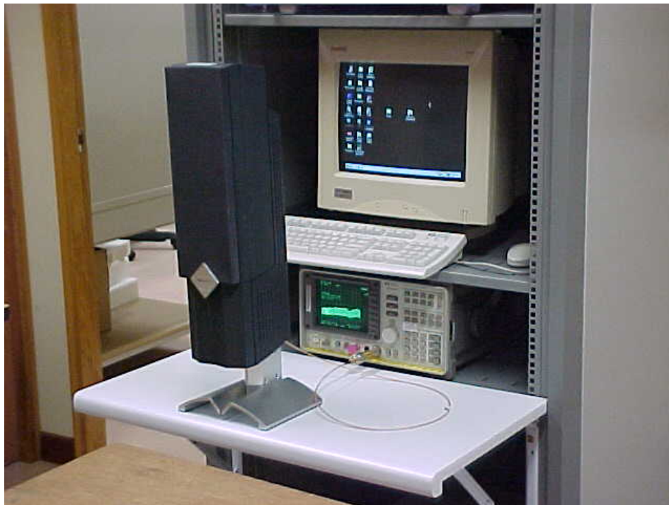
RF Conducted Spurious Emissions & Band Edge Compliance Measurement Test Setup – Wireless Speaker
