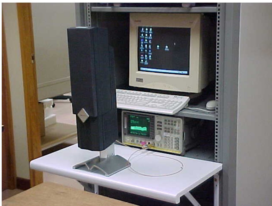
Spectrum Bandwidth Measurement Test Setup – Wireless Speaker
