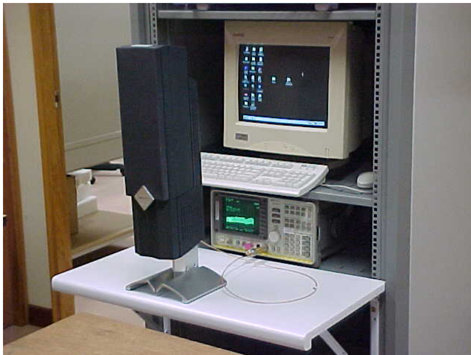
Average Frequency Dwell Time Measurement Test Setup – Wireless Speaker
