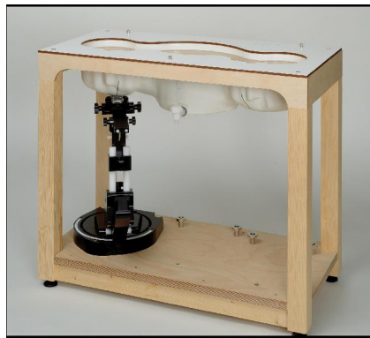
Picture C.10: SAM Twin Phantom
