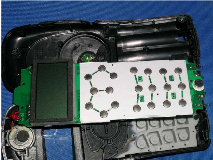
Handset Main PCB display side (View 1)
