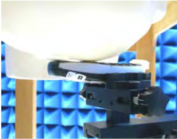
Figure 14.Right Head SAR Test Setup (Cheek)
