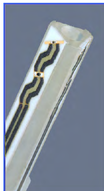
Figure 7. EX3DV3 E-field Probe
