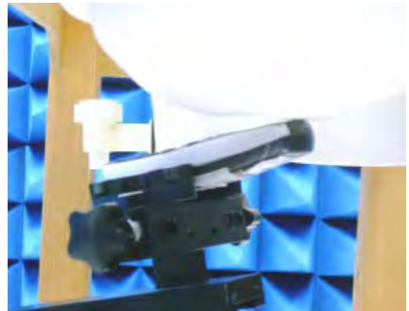
Figure 17.Left Head SAR Test Setup (Tilted)
