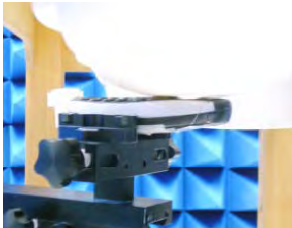
Figure 16.Left Head SAR Test Setup (Cheek)
