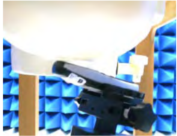
Figure 15.Right Head SAR Test Setup (Tilted)
