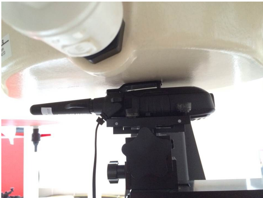
Body-worn, the front of the EUT towards ground with belt clip and Headset (The distance was 0cm)
