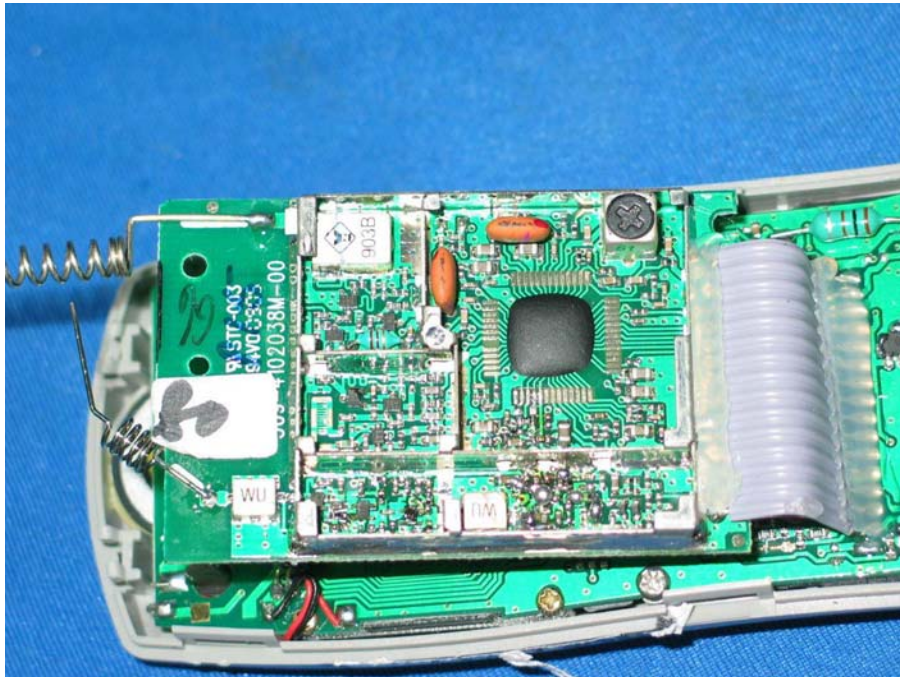
Handset Oscillator PCB comp side
