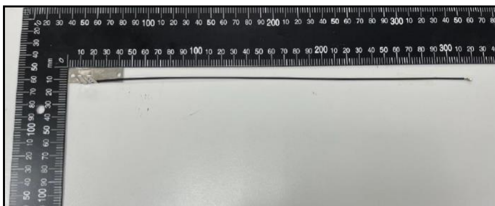
PIFA Antenna (Model: RFMTA421230IMMB701)
