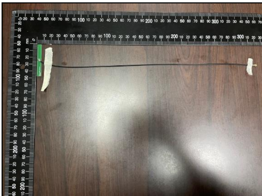
Dipole Antenna (Model: RFPCA460632IMMB701)
