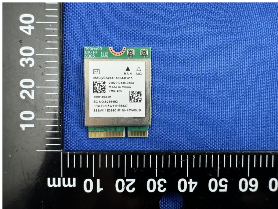
RF MODULE TOP VIEW-MT7925B22M(WITH SHIELDING)
