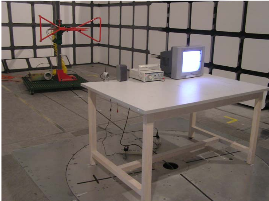
Radiated Emissions-Front View (below 1GHz)
