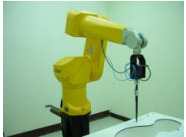
Fig. 5.2 Probe setup on robot
