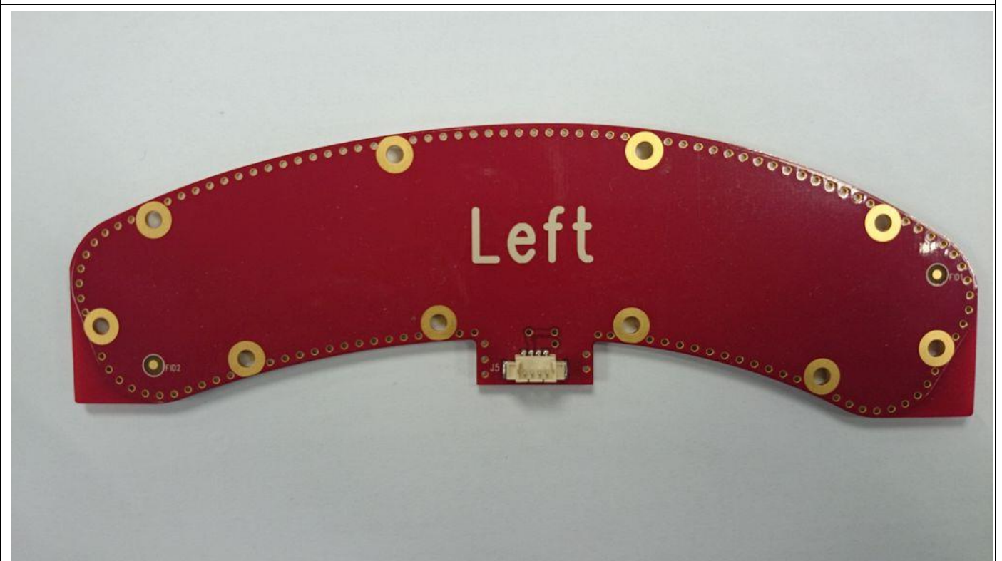
HALO LED PCBA – LEFT & RIGHT (LEFT SHOWN)
