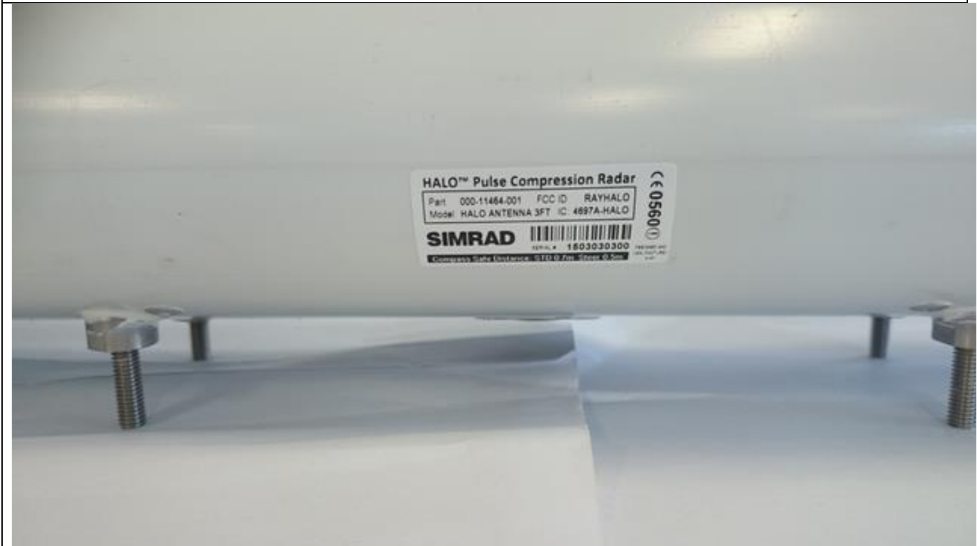
HALO Antenna – Serial Number label location
