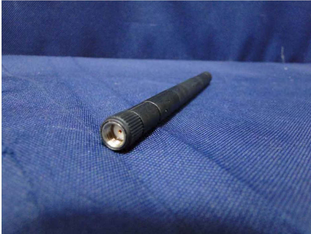
(11) EUT Photo _ Wi-Fi Antenna
