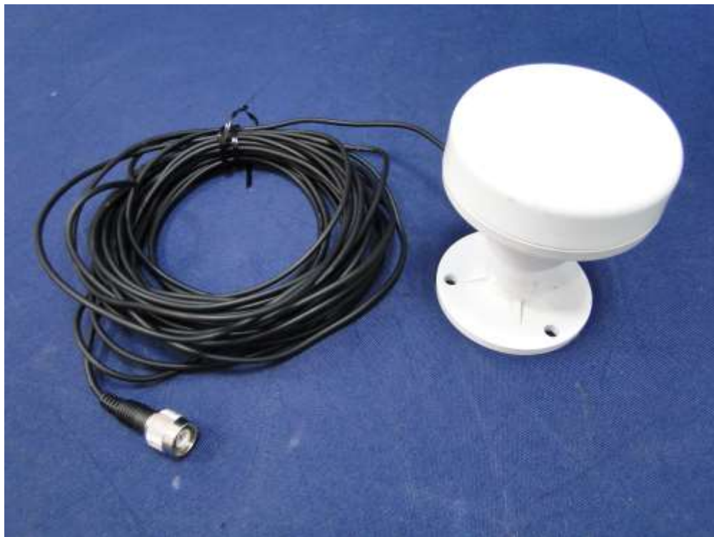
(8) EUT Photo _ GPS antenna with 10m Cable
