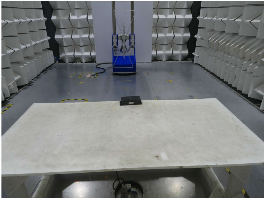
Radiated spurious emission Test Setup-1(Below 1GHz)
