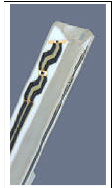
Inside view of ET3DV6 E-field Probe
