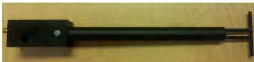
Figure 1 – MVG COMOSAR Validation Dipole
