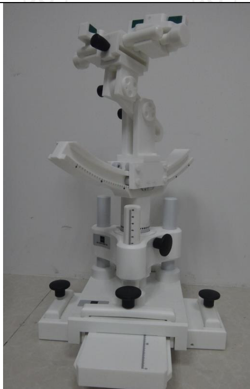
COMOSAR Mobile phone positioning system
