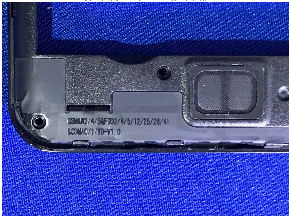
GSM&WCDMA&LTE Antenna View
