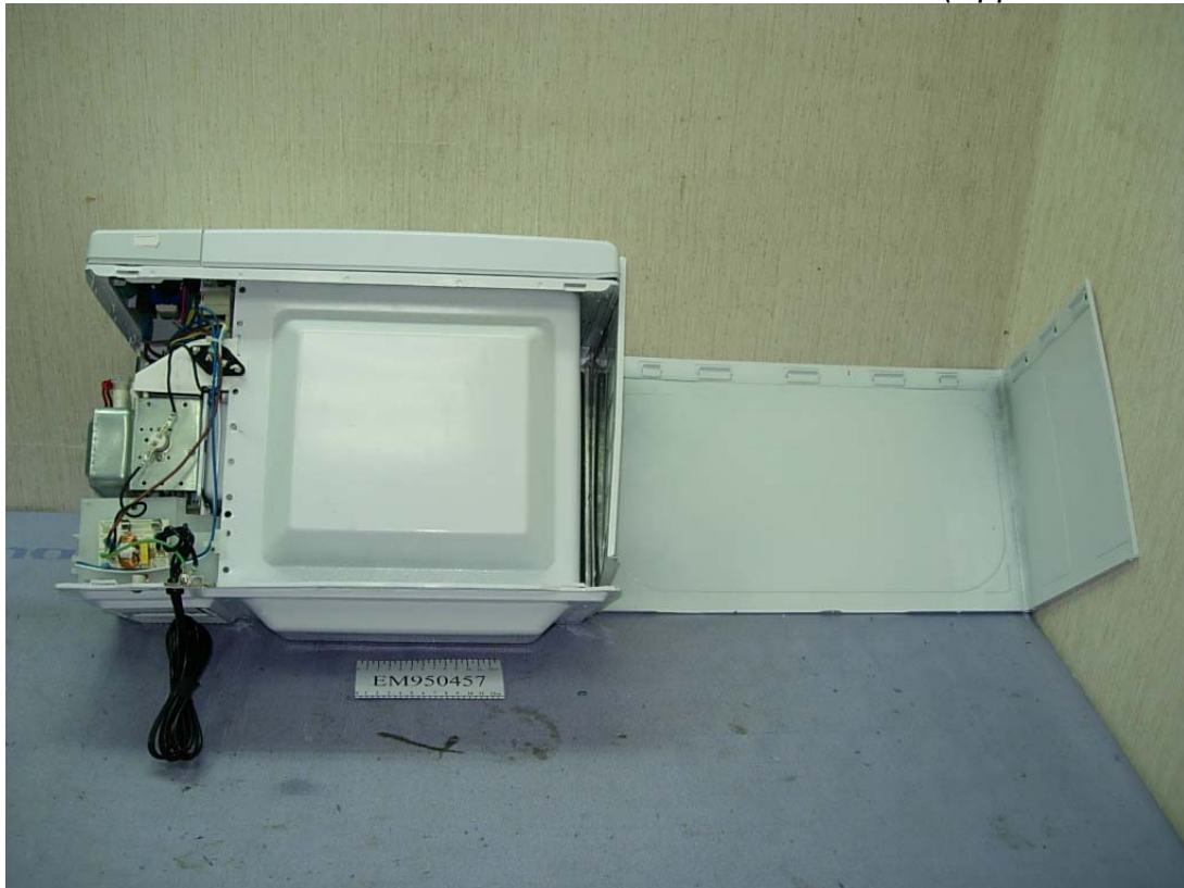
Photo 5 Internal View (Upper Cover Removed)
