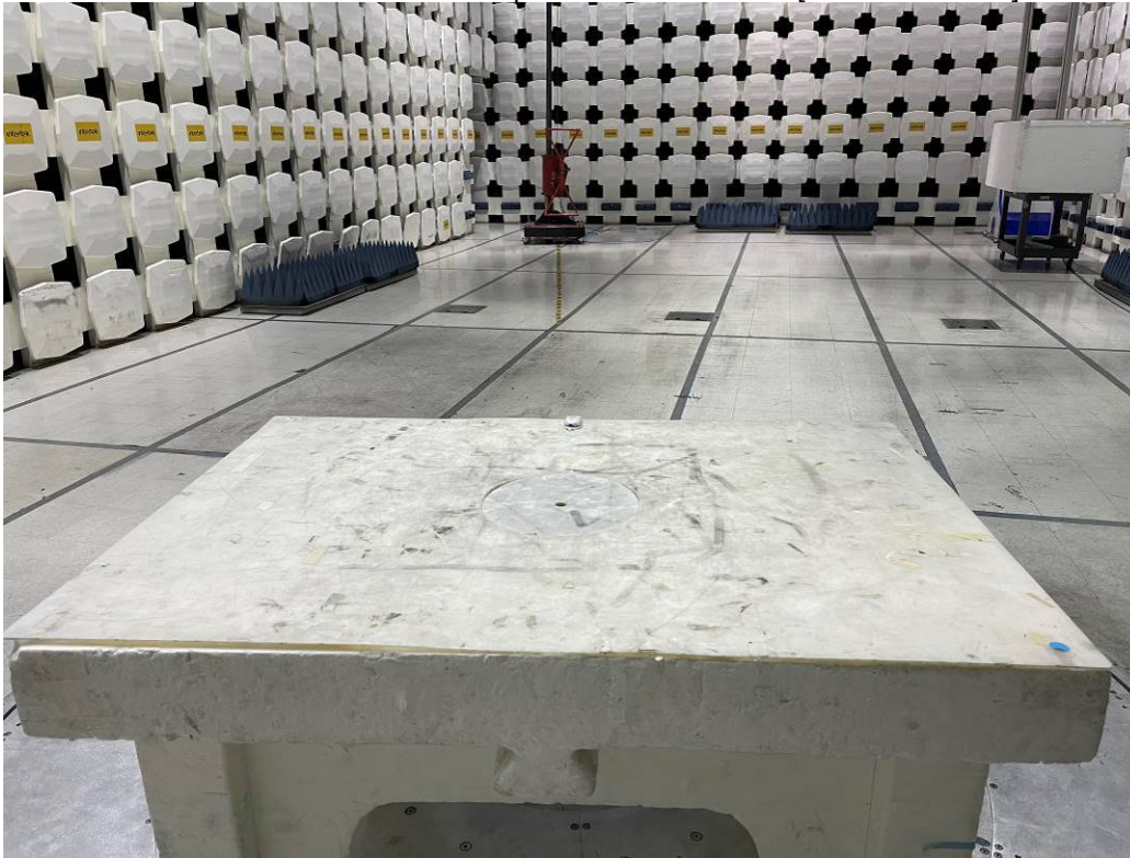
Radiated Emissions Test Setup From 30-1000 MHz [EUT on its back]
