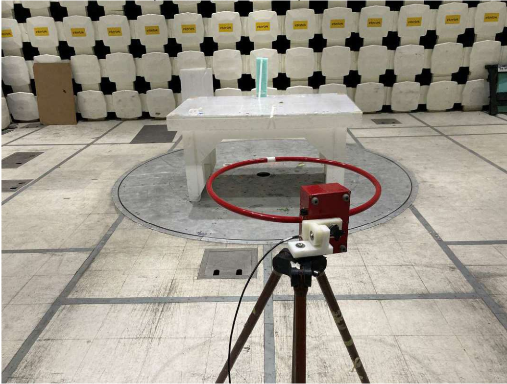
Test Setup, RE 9kHz-30 MHz, Loop antenna on Z-Axis
