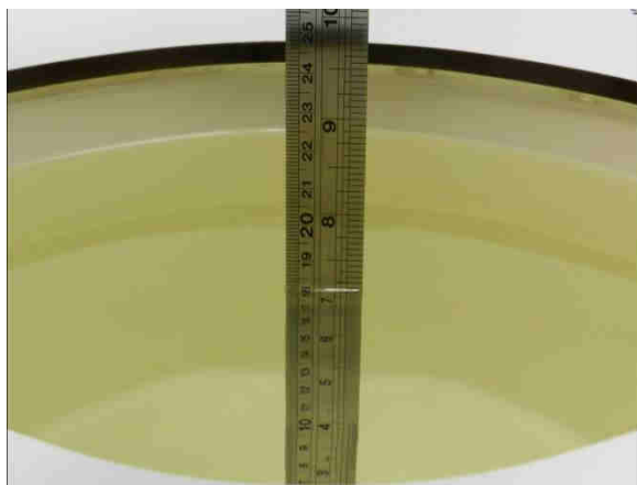
Fig 10.1 Photo of Liquid Height for Body SAR
