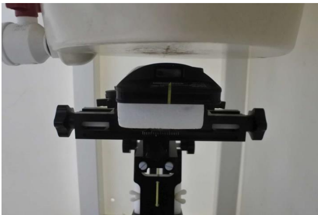
Back, Test Separation 13 mm
