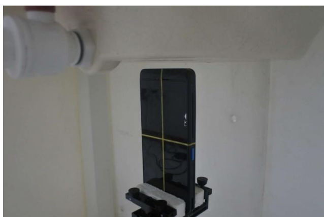
Top Side, Test Separation 10 mm
