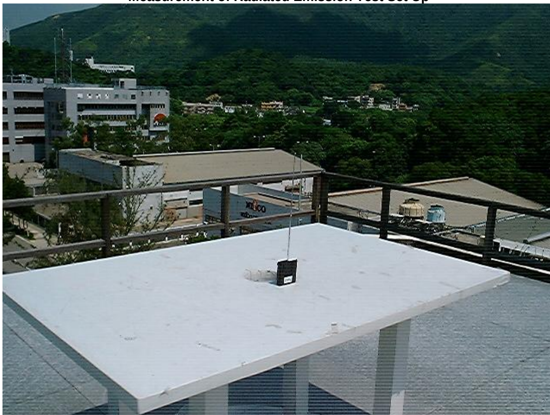
Measurement of Radiated Emission Test Set Up
