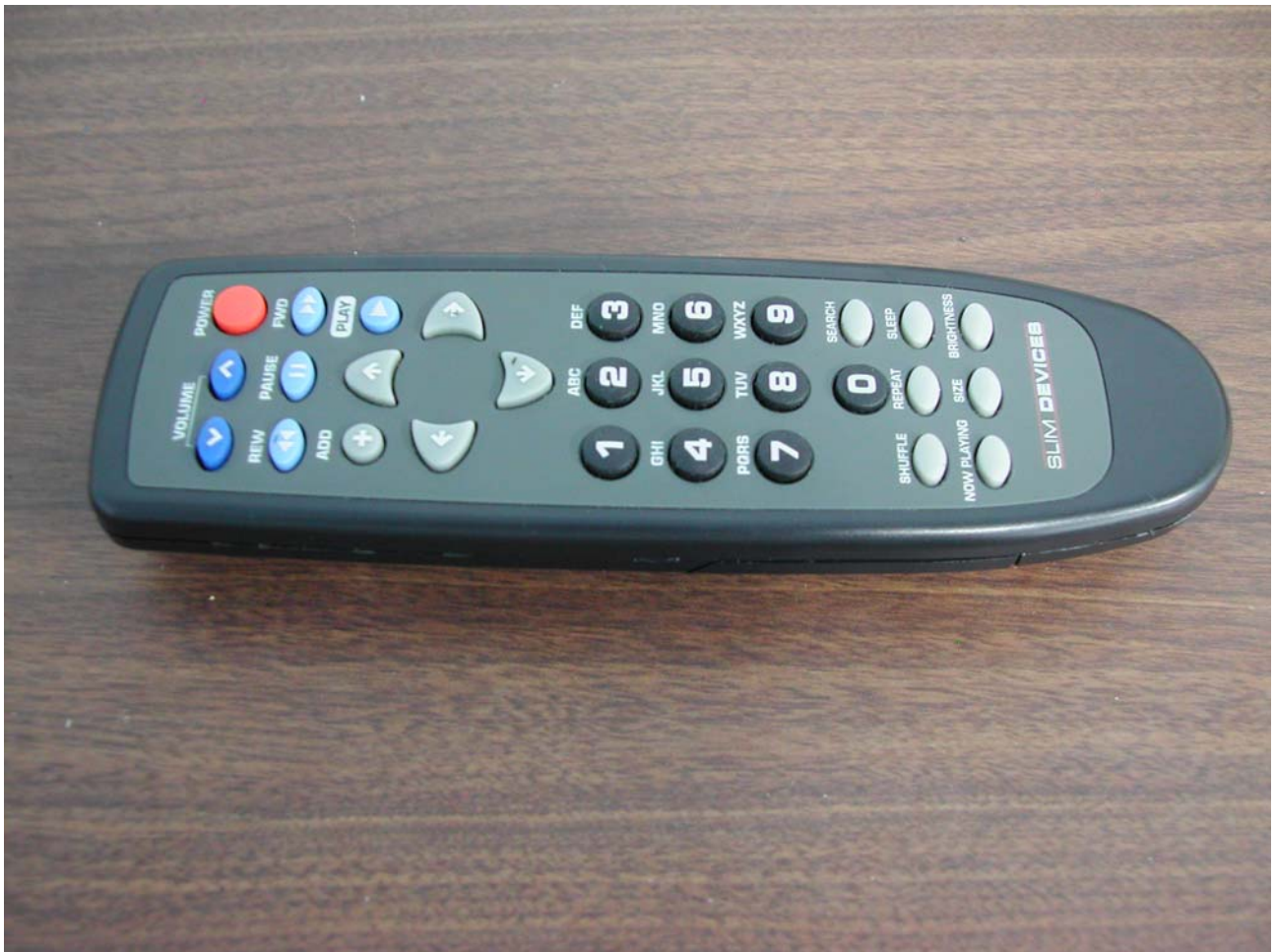
FIGURE 6: PLI Photograph Number 5392C2633SJ-17 illustrates the Slim Devices Remote Control, model SC33 used to operate the Squeezebox.
