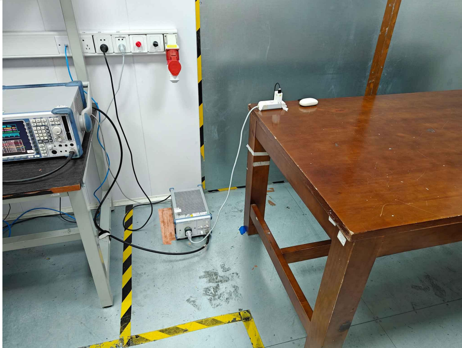
Conducted emissions at AC power line (150kHz-30MHz)
