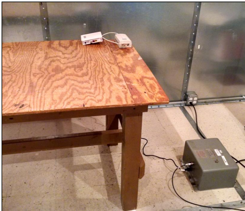
Photograph 2. Conducted Emissions, Test Setup, PoE
