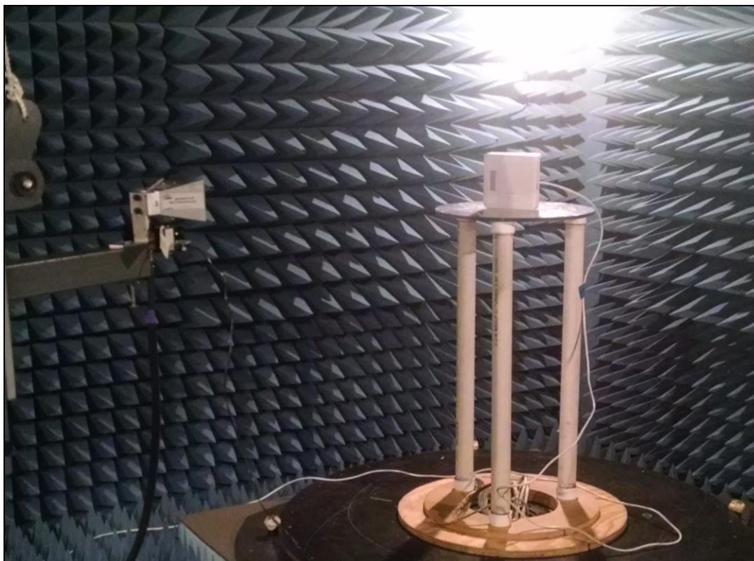
Photograph 7. Radiated Spurious Emissions, Test Setup, 18 MHz – 40 GHz
