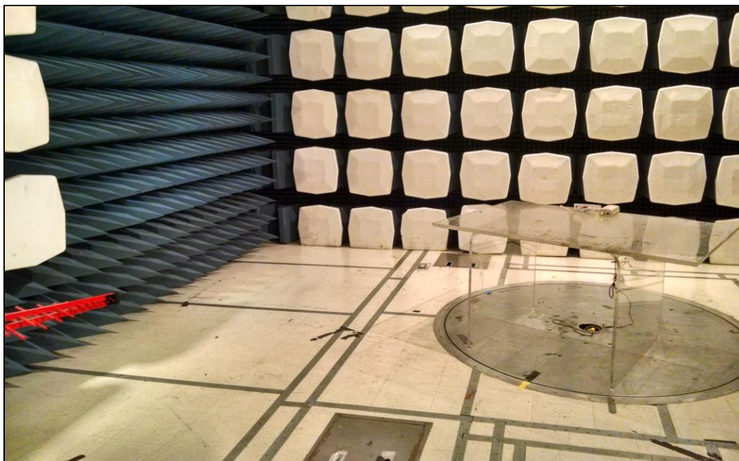
Photograph 5. . Radiated Spurious Emissions, Test Setup, 30 MHz – 1 GHz
