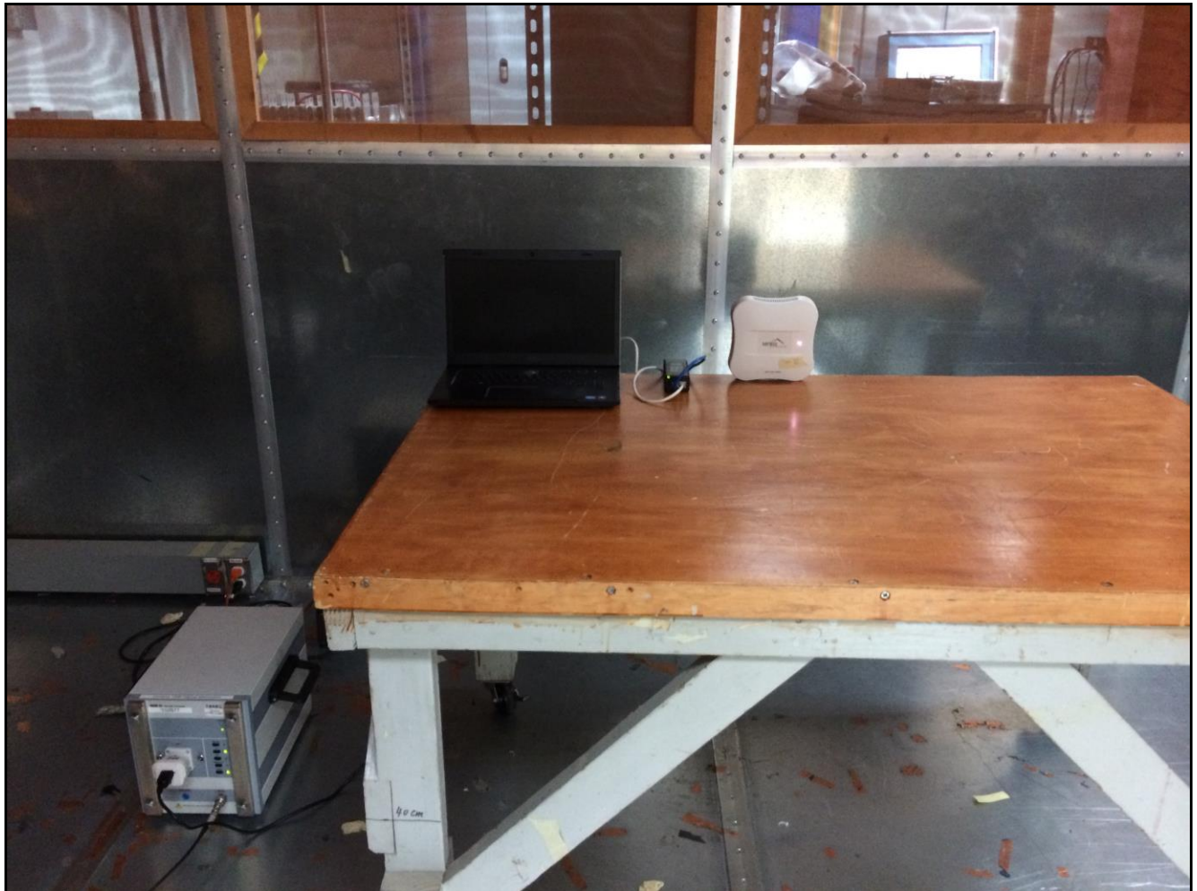
Photograph 2. Conducted Emissions, 15.207(a), Test Setup
