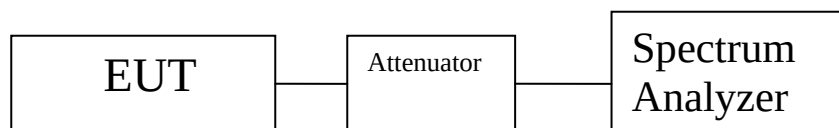
Figure 5. Peak Excursion Ration Test Setup
