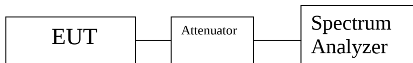
Figure 2. Block Diagram, Occupied Bandwidth Test Setup
