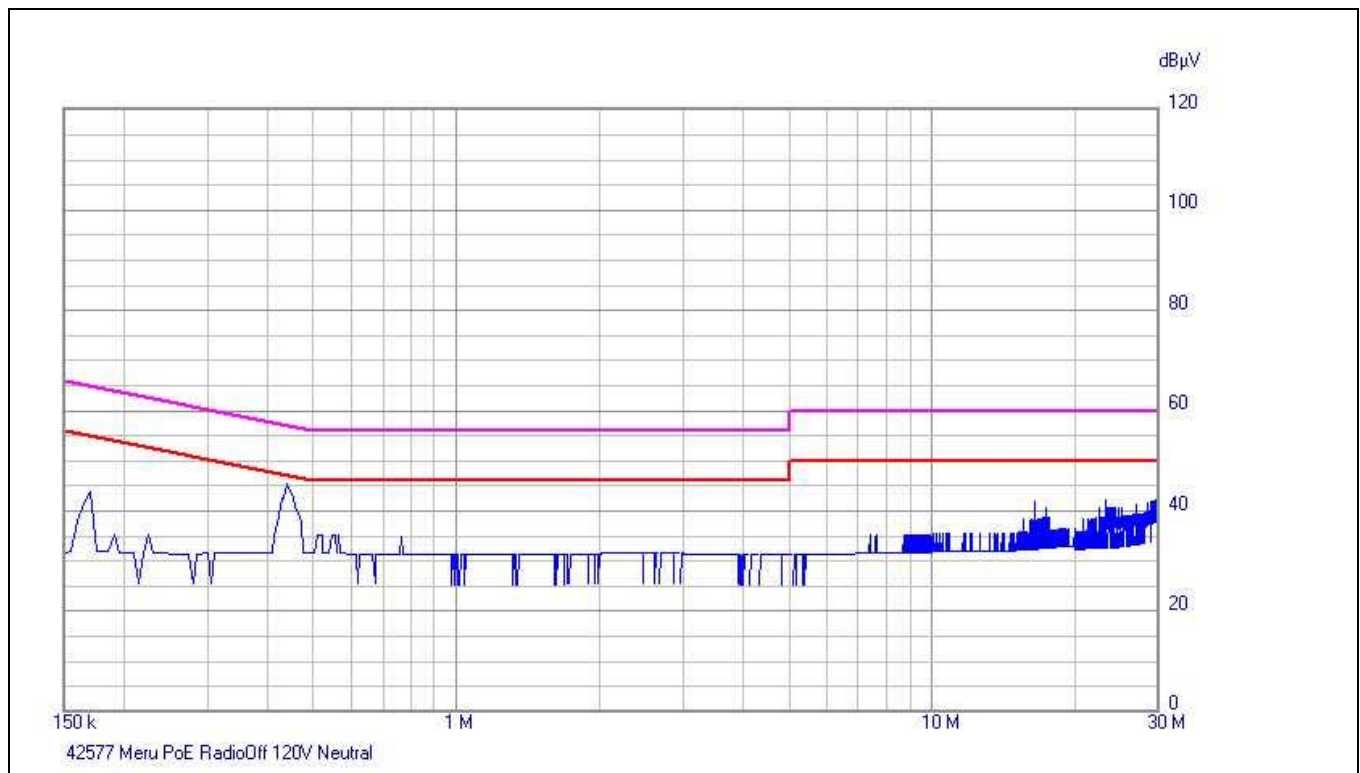
Plot 2. Conducted Emissions, Neutral Line, PoE
