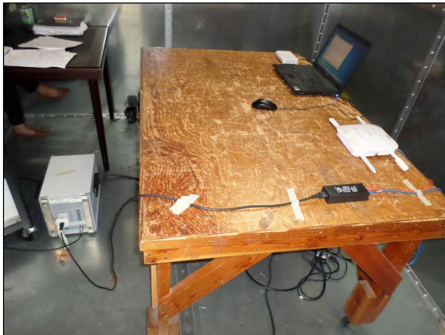
Photograph 2. Conducted Emissions, Test Setup, PoE
