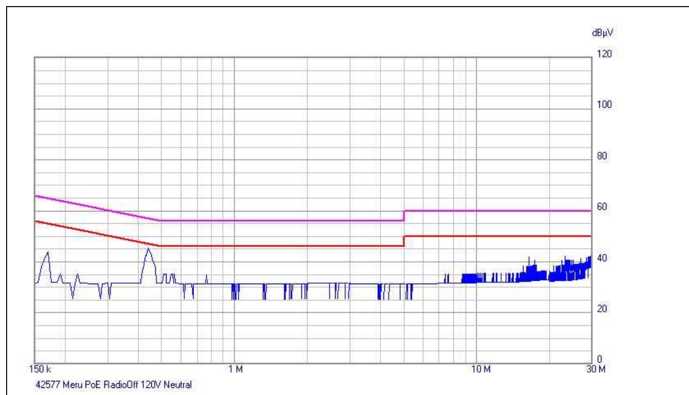
Plot 10. Conducted Emissions, 15.207(a), Neutral Line, PoE
