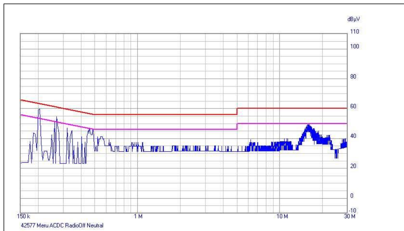
Plot 12. Conducted Emissions, 15.207(a), Neutral Line, AC/DC
