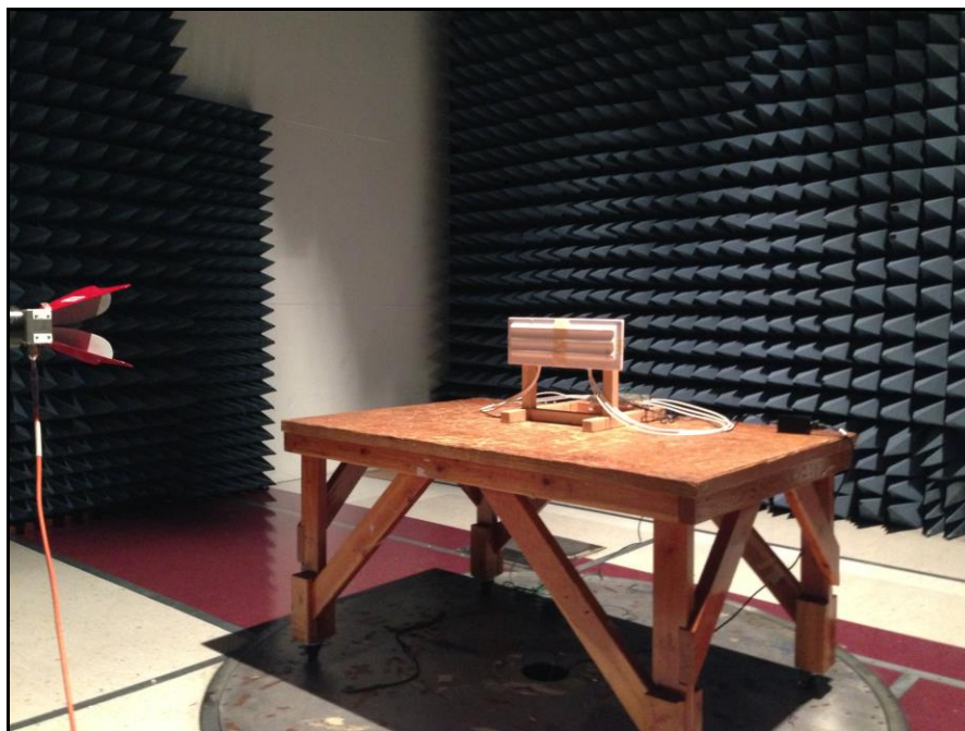
Radiated Spurious Emissions, Patch Antenna, Test Setup, 1 GHz – 18 GHz
