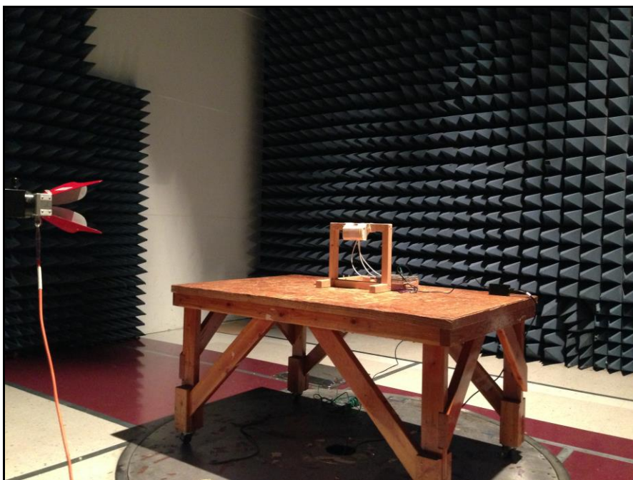
Photograph 7. Radiated Spurious Emissions, Ceiling Antenna, Test Setup, 1 GHz – 18 GHz
