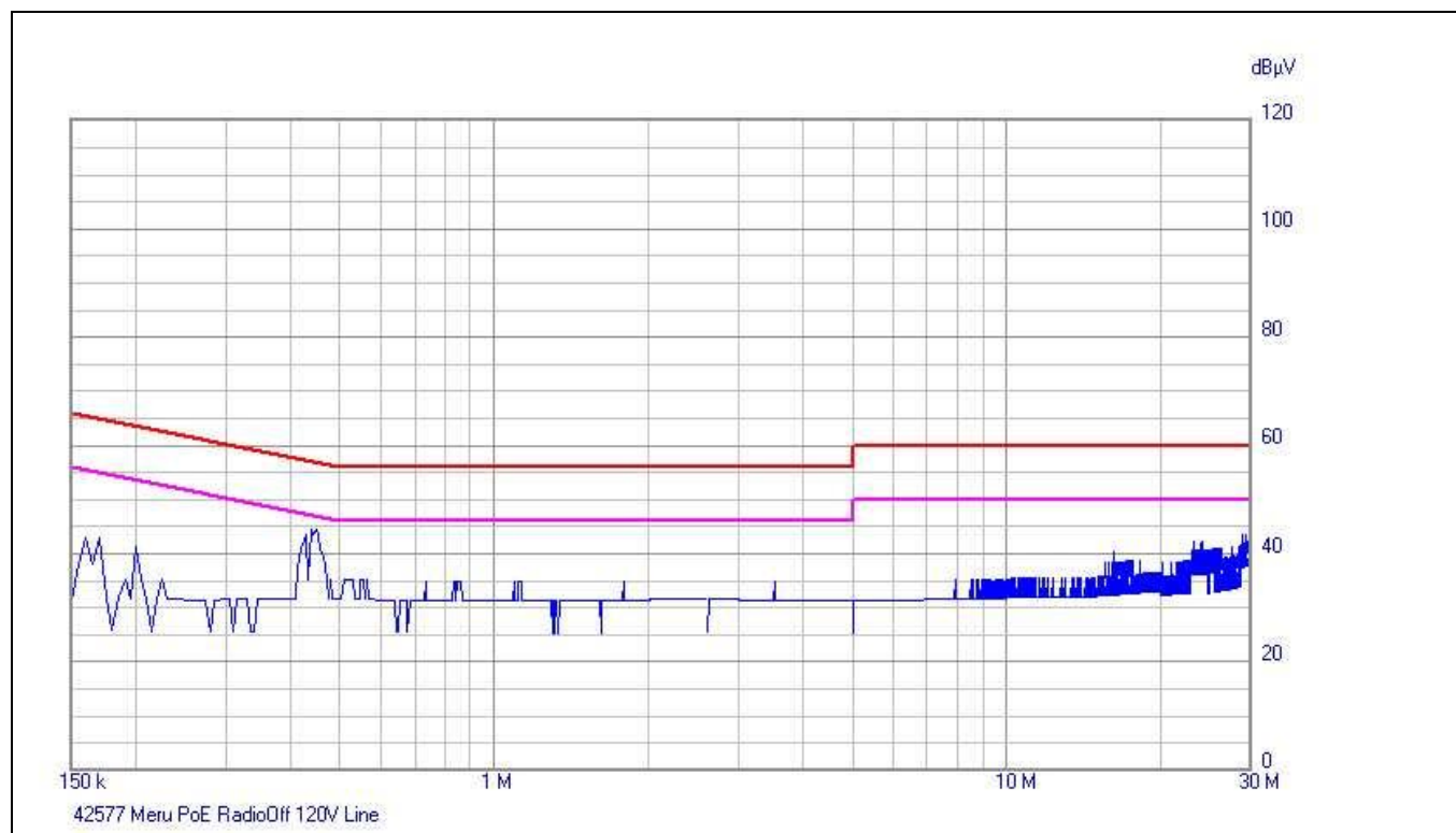
Plot 9. Conducted Emissions, 15.207(a), Phase Line, PoE
