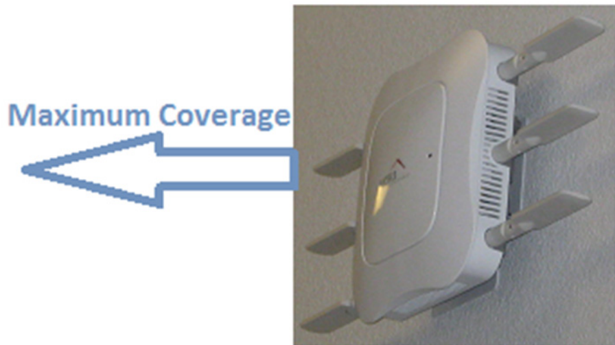
Figure 14: Horizontal Antenna Orientation (Side View)
