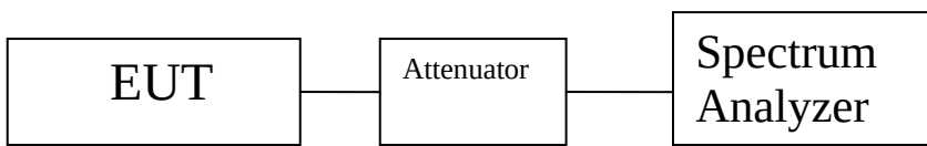
Figure 3. Power Output Test Setup
