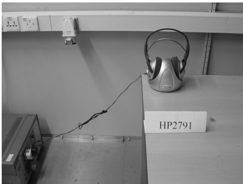
Photograph 1: Set-up for Conducted Emission on AC Mains
