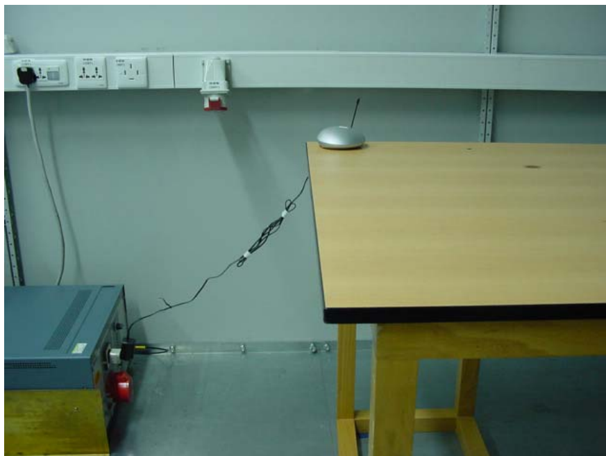
Photograph 2: Set-up for Radiation Measurement Below 1GHz
