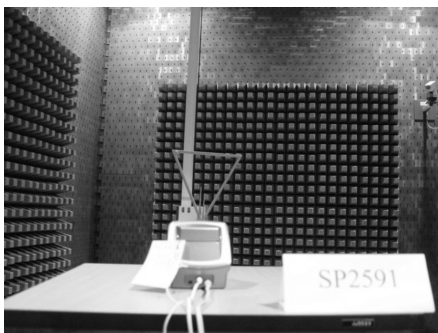
Photograph 2: Set-up for Radiation Measurement Below 1GHz
