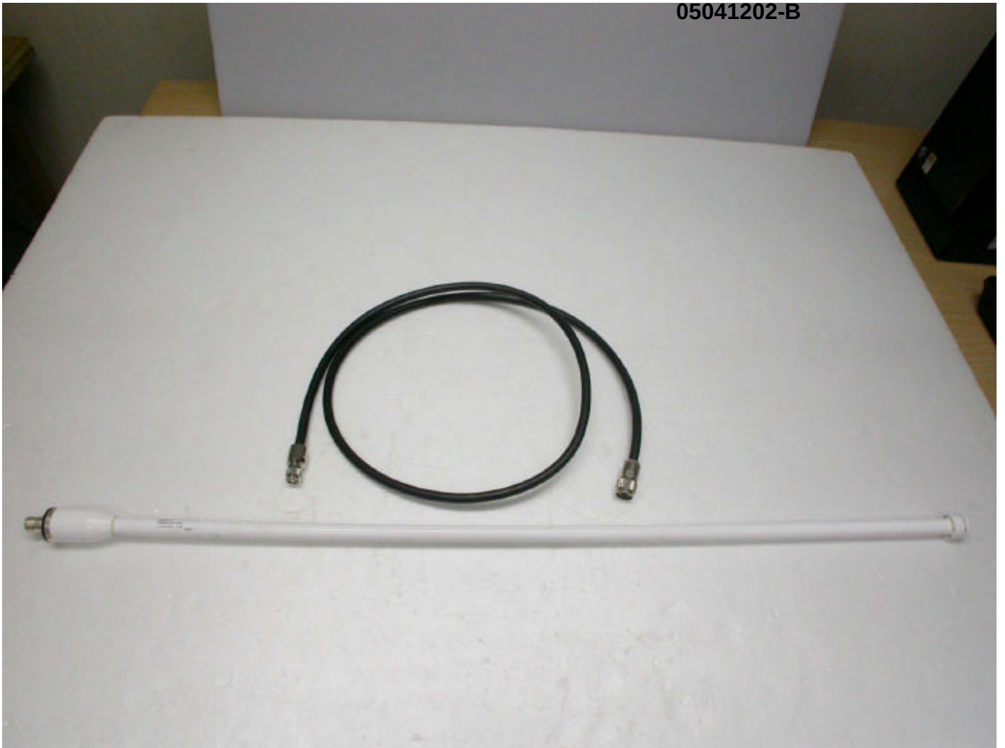
External omni antenna (model: MFB24010)
