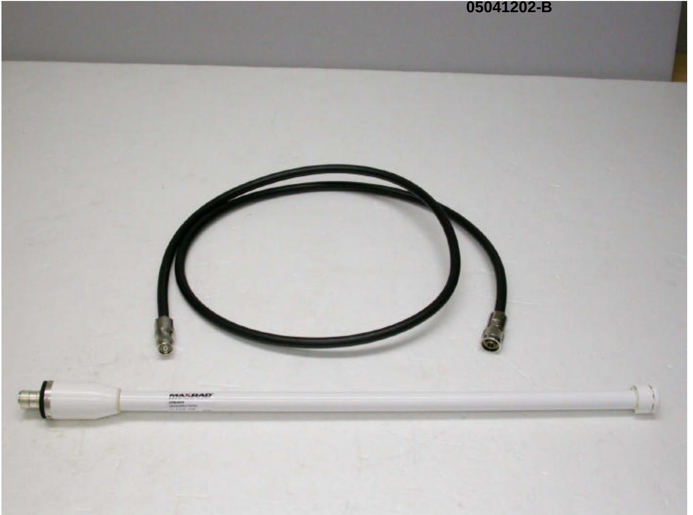
External omni antenna (model: MFB49009)
