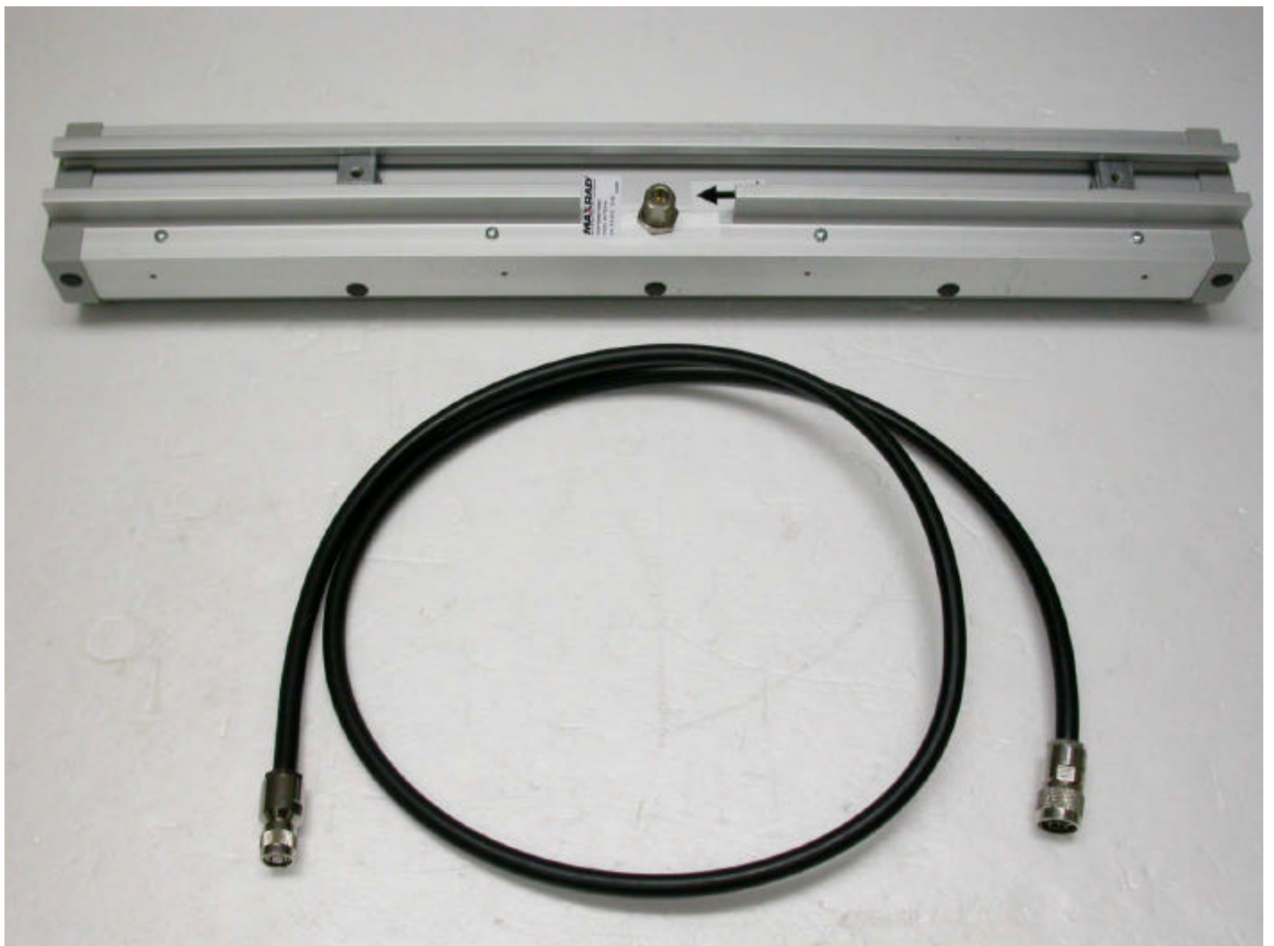
External sector antenna (model: WISP4959018MBV)
