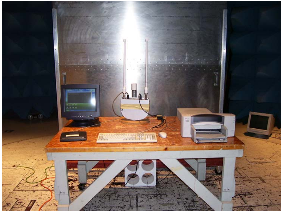
Photograph 2. Conducted Emissions Test Setup
